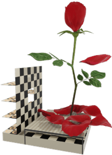
Figure 7: A Dronevision (DV) with charging stations behind a wall at the back of the display. FLSs with depleted batteries fly through the narrow vertical opening to land on a charging station and charge their batteries.
